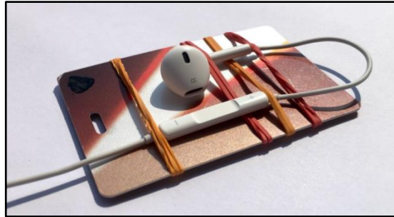
Figure 2: Example setup for holding the earpiece and microphone
